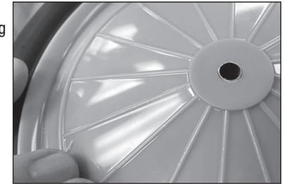
6. Secure the wheels to the main axle using the wheel collars and M3 x 3 setscrews. The wheel collars are placed on either side of the wheel. Make sure to use a file to make a flat area on the main axle for the setscrews. Apply a drop of threadlock on each setscrew before tightening them using a 1.5mm hex wrench.
