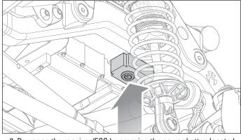
8. Power on the receiver/ESC by pressing the power button located on the bottom of the chassis, opposite the steering servo.
